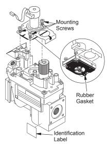
Figure 59 - Installing Pressure Regulator Assembly
